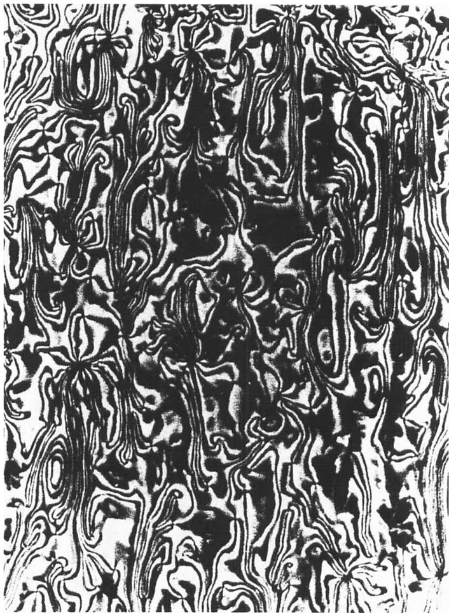
FIGURE 6 4,4'-tetradecanoyloxybenzalazine. T = 407.0 K; smectic liquid; crossed polarizers.
